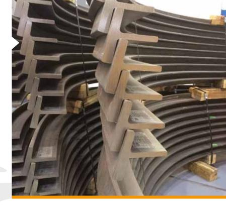
Aries Manufacturing has developed a very innovative Hot Stretch Forming process to contour titanium profiles for airframe component applications.
