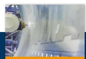
Typical parts produced with MMS°: fuselage aluminum 3D skins to perform pocketing, drilling a routing in a single setup.
