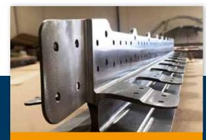
Typical parts produced with Hot Stretch Forming: Titanium airframe components
